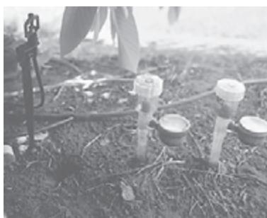
Figure 26. Tensiometers in place, (a) in major root zone and (b) below most roots
