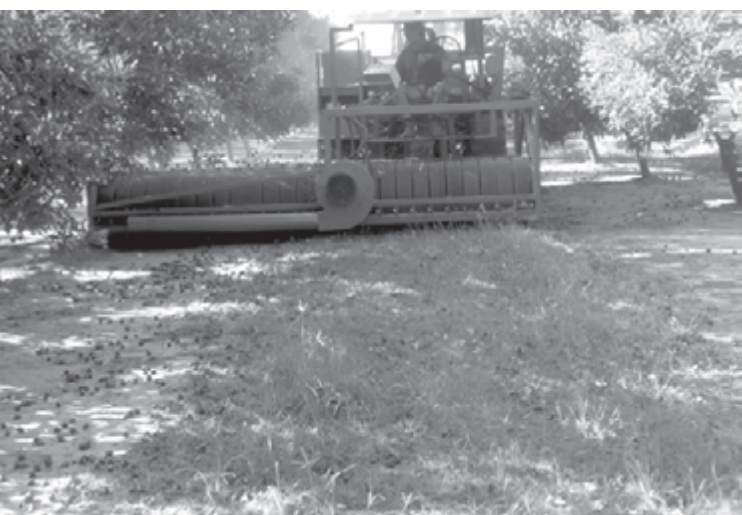
A large finger wheel harvester. Note that the larger harvesters use blowers to remove nuts from under the trees
